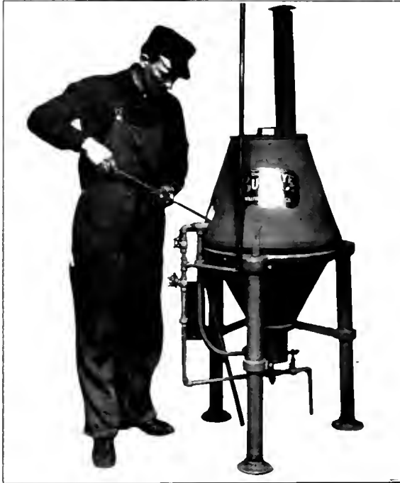
Files Being Cleaned in a Buckeye Machine
